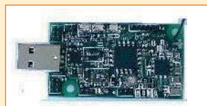
One of Cratlons products - C701EM1 .. Zigbee™-ready 802.15.4 MSP430 Wireless Sensor module & Development Board
